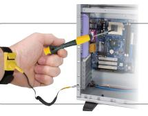
1. It sends all body static charge to the ground, suitable to work with delicate electronic devices without any risk of damage.
